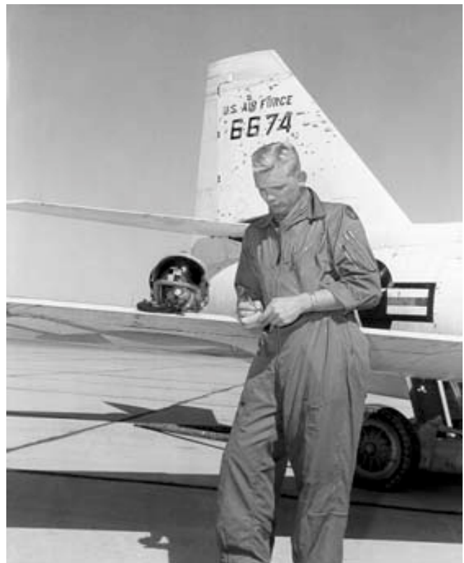
Capt. Iven Kincheloe and X-2 is pictured here following a high speed research flight. Note heat-blistered paint on vertical tail.
